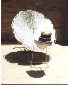
1.5m 2 Scheffler cooker with fixed focus – notice 2 pots
