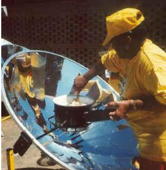
A project consultant tends to a dish in an SK12 parabolic cooker
