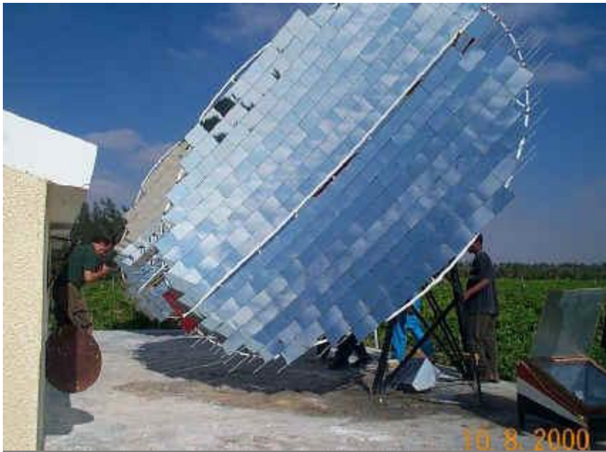
Individual mirrors attached to a parabolic frame
