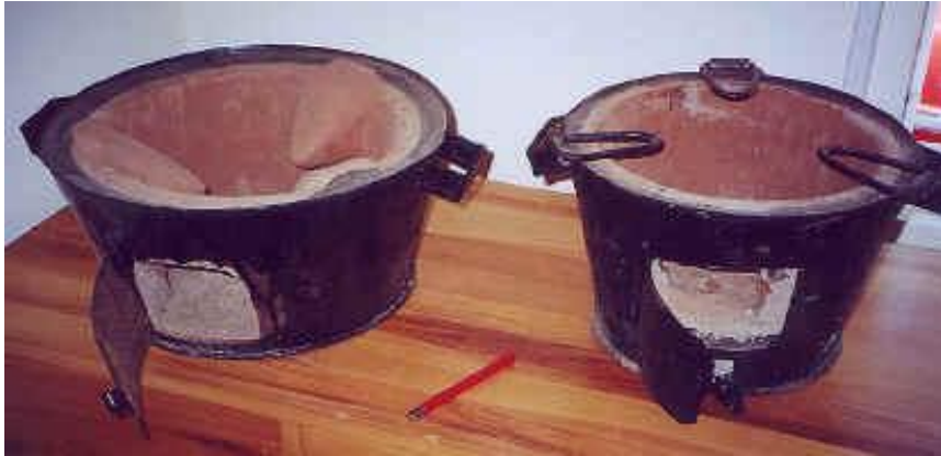
Fuel-efficient wood stoves with locally-crafted ceramic linings
