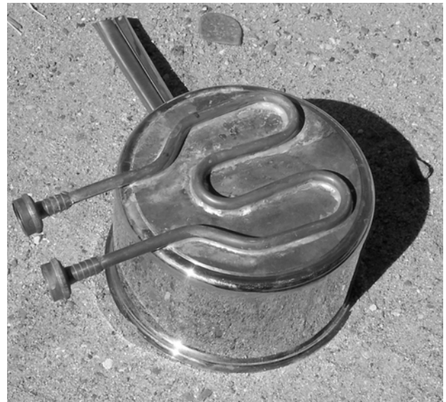
Fig.3. Heat Exchanger Detail. Disconnect fittings were eliminated after initial testing in favor of non-removable Hotplate installation.
